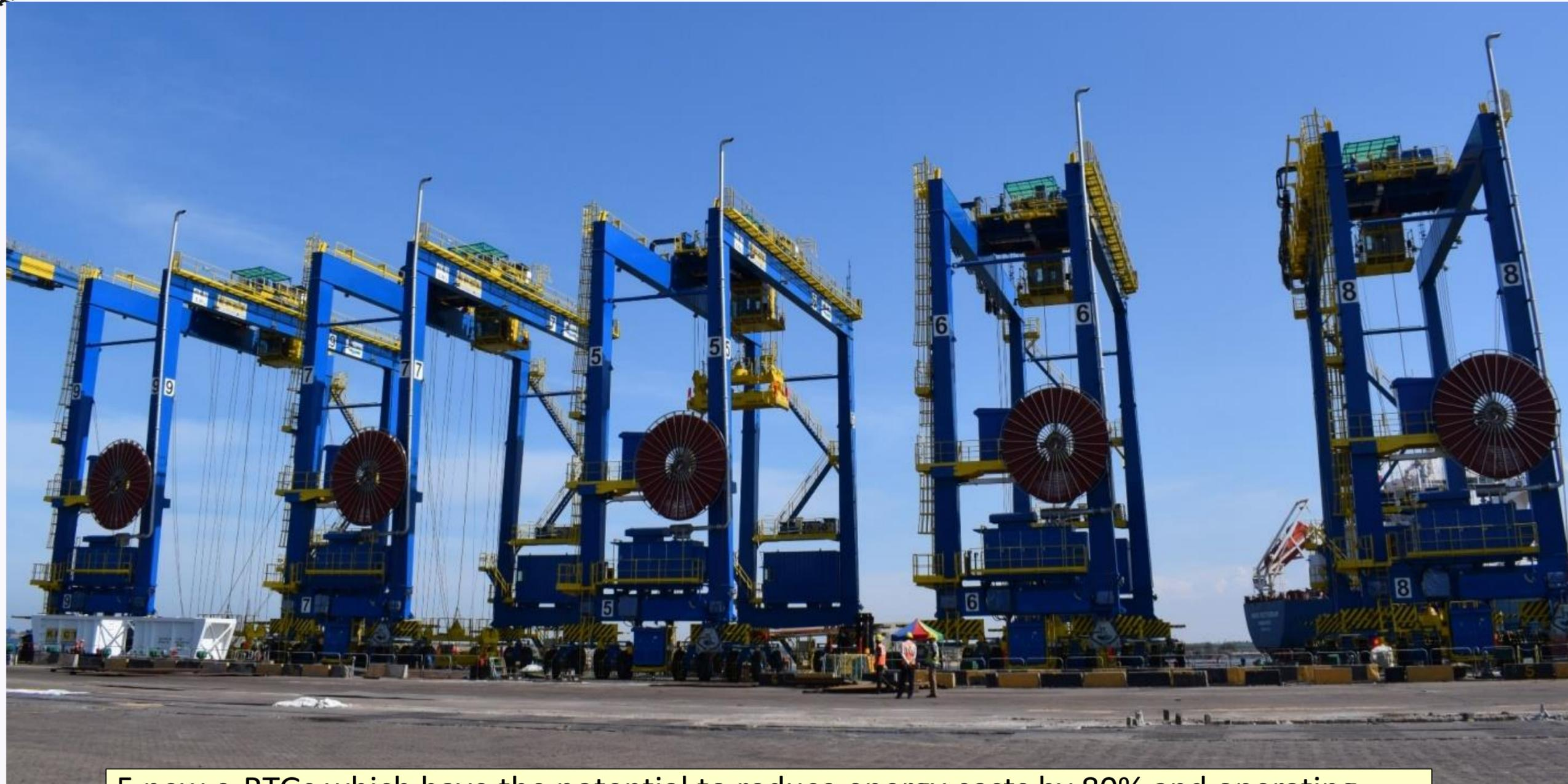
5 new e-RTGs which have the potential to reduce energy costs by 80% and operating noise level by 65% whilst cutting down more than 1400 tonnes of Greenhouse Gases (GHG) emissions vis-à-vis the traditional diesel run RTGs.
